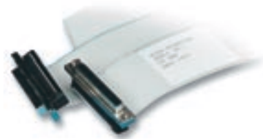
Figure 20. R6868 Ribbon Cable
