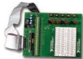
Figure 4. SC-2075 Breadboard Connector Block
