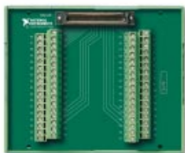
Figure 4. TBX-68 I/O Connector Block
