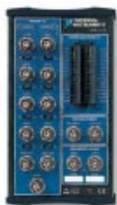
Figure 1. BNC-2110 I/O Connector Block
