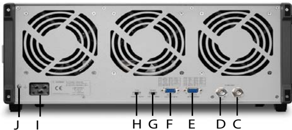
Figure 1-6: PXES-2780 Rear Panel Connectors
