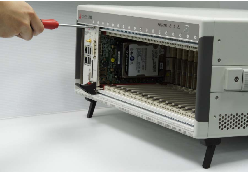
Figure 2-5: Fasten System Controller Module Screws
