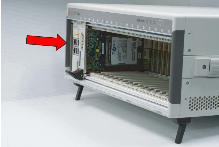
Figure 2-3: Align System Controller Module
