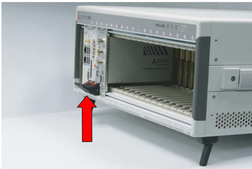
Figure 2-7: Secure Peripheral Module Latch
