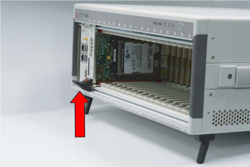
Figure 2-4: Secure System Controller Module Latch
