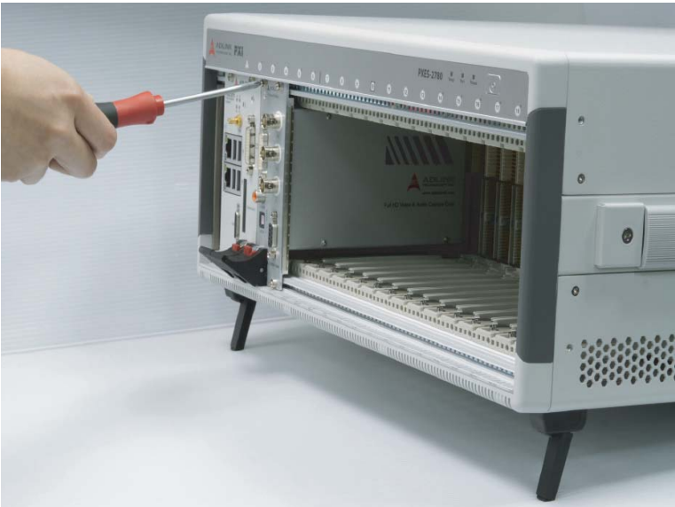
Figure 2-8: Fasten Peripheral Controller Module Screws
