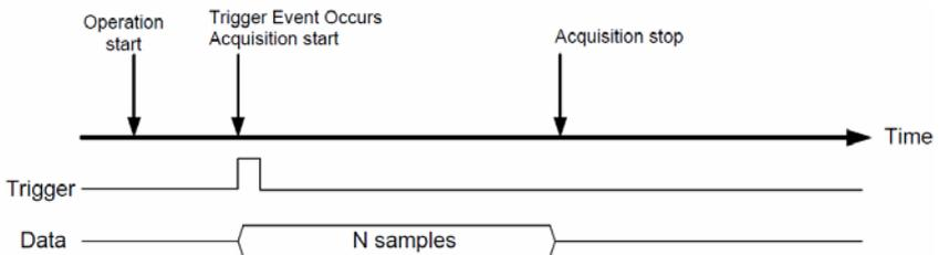
Figure 3-5: Post-Trigger Acquisition
