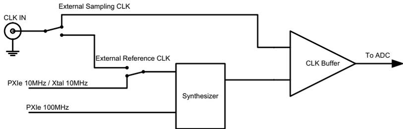
Figure 3-10: PXIe-9852 Clock Architecture
