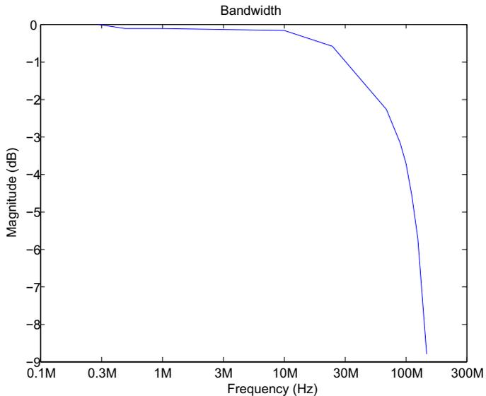
**Figure 1-1: Analog Input Channel Bandwidth,  $\pm 0.2 V_{pp}$**
