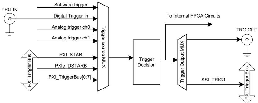
**Figure 3-3: Trigger Architecture of the PXIe-9852**
