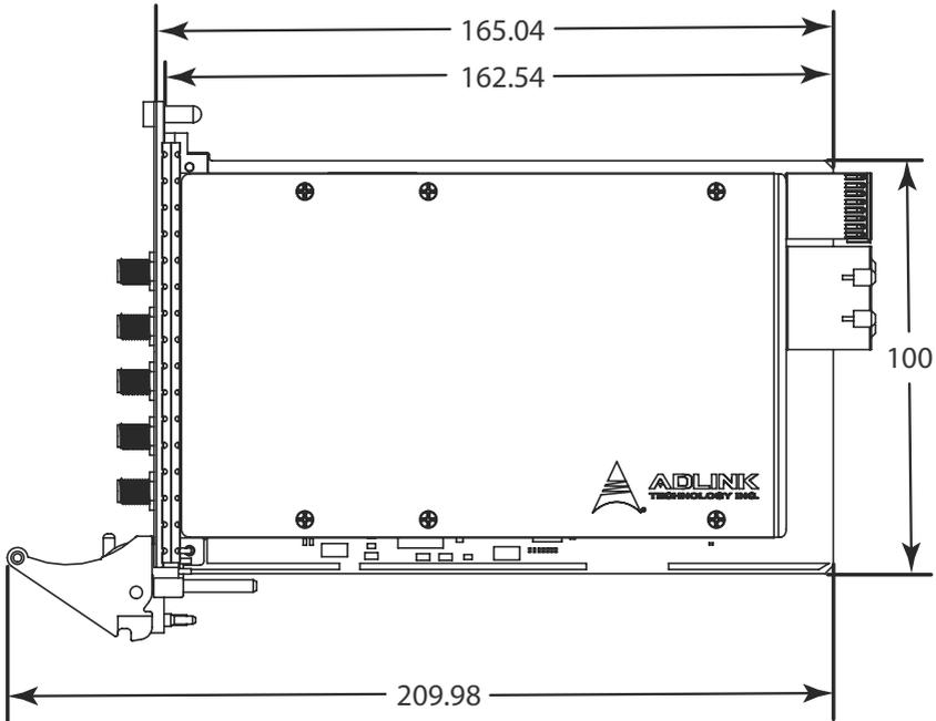
Figure 1-3: PXIe-9852 Schematic
