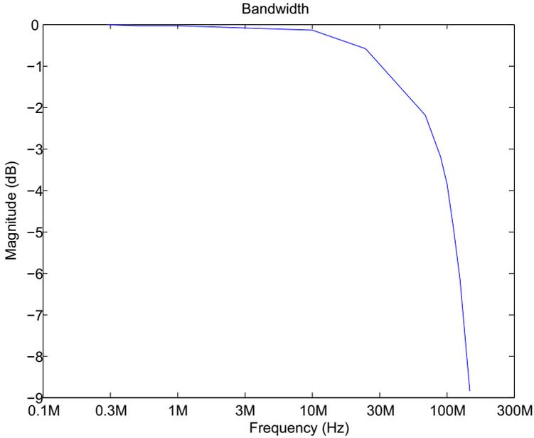
**Figure 1-2: Analog Input Channel Bandwidth,  $\pm 2$  Vpp**
