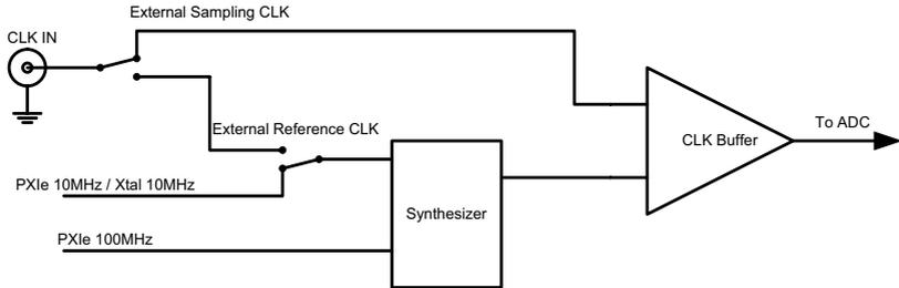
Figure 3-10: PXIe-9852 Clock Architecture
