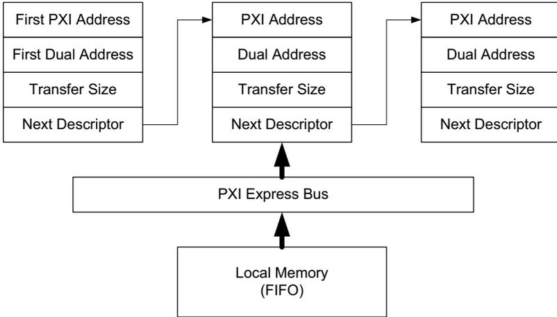
**Figure 3-2: Linked List of PCI Address DMA Descriptors**
