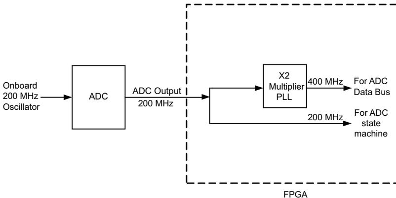
Figure 3-11: PXIe-9852 Timebase Architecture
