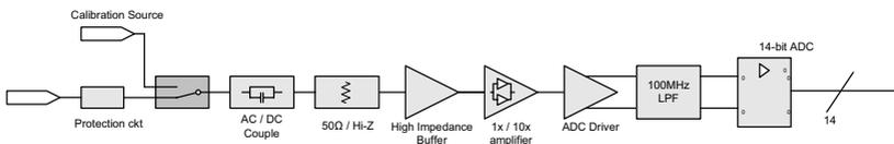
Figure 3-1: Analog Input Architecture of the PXIe-9852
