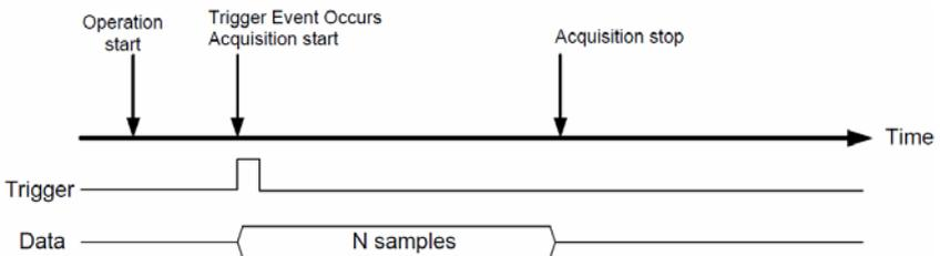
Figure 3-5: Post-Trigger Acquisition
