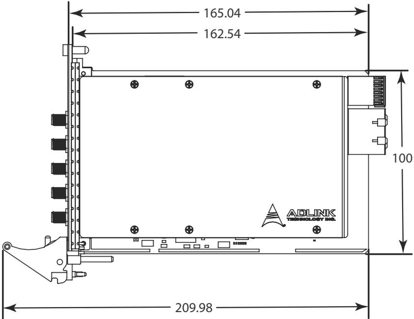
Figure 1-3: PXIe-9852 Schematic
